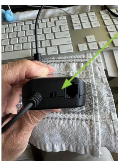
There is a volume control on this device and you can turn it all the way left or right. Recommend turning it about half way and then leave it alone as you will be using the volume control on the PC that this is hooked up to.
